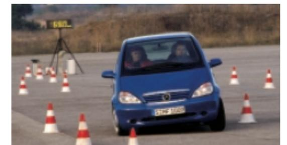
top secret "Elk test" drive of the newly modified A-class car – a test of immense importance for Mercedes-Benz (the earlier car flipped over in a test maneuver done by a Swedish car magazine).
